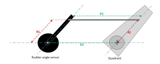
Picture1: installation of a nke rotary rudder angle sensor
